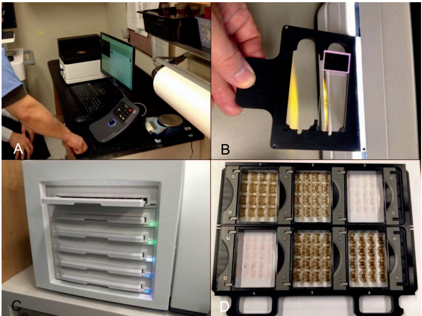
Figure 4. A, Frozen section room is shown with a small desktop WSI scanner that does not occupy much counter space. B, A low-volume scanner is shown with a slide tray that holds only 2 glass slides. C, High-volume WSI scanner that allows multiple slides to be loaded by using slide trays. D, Huron WSI scanner tray (Huron Digital Pathology, Waterloo, Ontario, Canada) that can accommodate large glass slides from whole-mount sections. Abbreviation: WSI, whole slide imaging.
