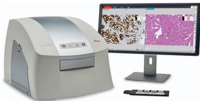
Figure 6. Aperio LV1 whole slide imaging scanner (Leica Biosystems, Vista, California) with robotic control allows users to remotely access live slides. Users can remotely switch between 4 slides, move slides in x- and y-axes, change magnification (between \times 2.5 , \times 10 , \times 20 , and \times 40 objectives), and adjust the fine focus (image courtesy of Leica Biosystems).
